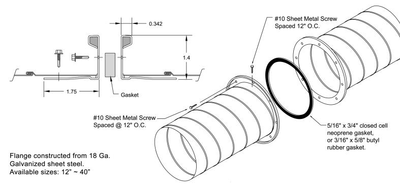
The use of the DuraFlange connecting system, installed and sealed per manufacturer's recommendations, is suitable for use on all systems across a range of internal duct pressure classes; from positive 10" S.P.W.G. to negative 10" S.P.W.G.
