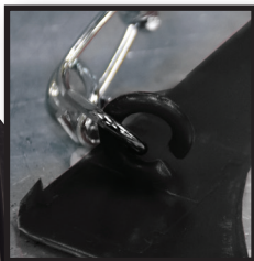
Loop inside lid keeps end of chain from getting lost
